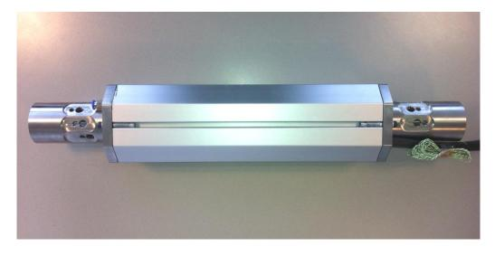
A linear motor-generator based around Libertine's flux switching machine architecture for motion control development and other research applications. The electrical machine can be operated using a linear encoder or a range of alternative sensor inputs.
