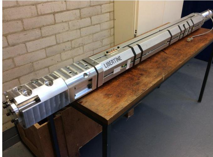
A free piston gas expander flux designed for high expansion ratio thermodynamic cycle research applications. The flux switching electrical machine is integrated with a passive inlet valve mechanism and a pneumatic preload system to accommodate a wide range of test conditions and objectives.
