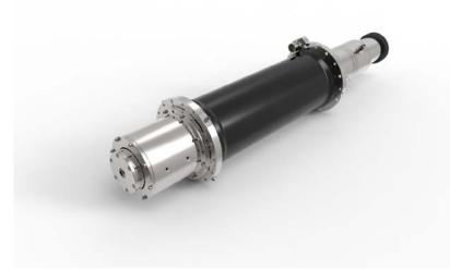
A high performance slotless linear electrical machine designed for high frequency dynamic testing applications. The electrical machine is integrated with low friction gas bearings and a pneumatic preload system to accommodate a wide range of test conditions and objectives.
